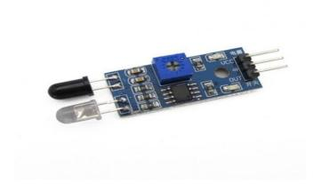
Fig -4: IR Transmitter and receiver sensor
